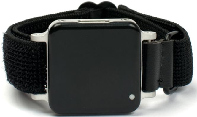
Movement monitors combine a number of sensors within a single package, including a 3 axis accelerometer, a 3 axis gyro, a 3 axis magnetometer, and a temperature sensor. The accelerometers can be configured in a high 6G mode, or a low 2G mode depending on the testing requirements. There are a number of options for securing the monitors on subjects using a selection of straps.
